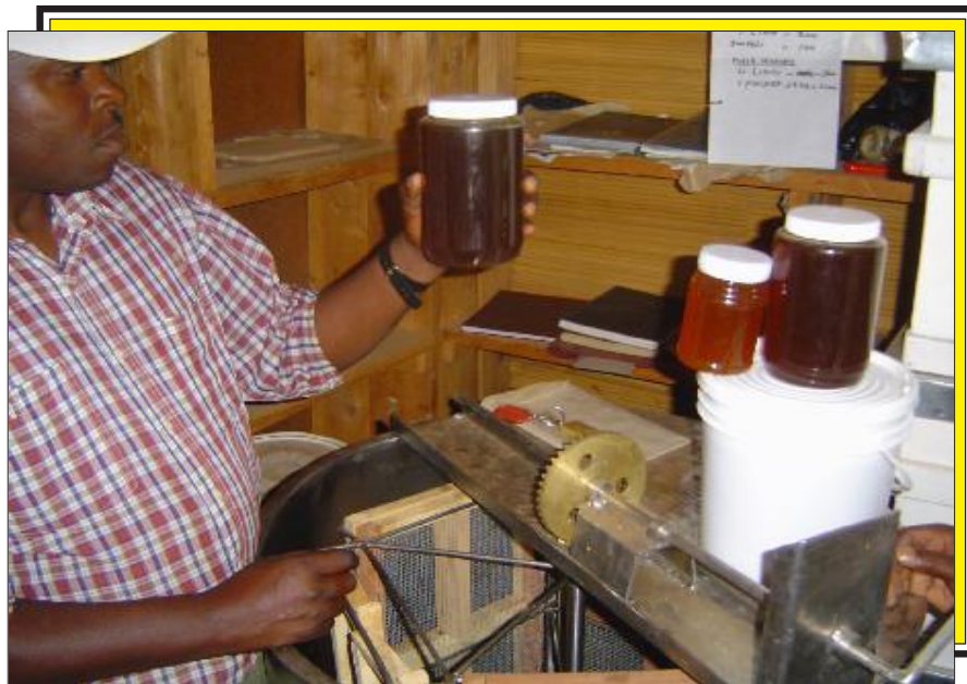
Photo 39: Centrifuge Centrifuge that handles honey from the KTBH (in wire baskets) as well as frames from the Langstroth hive.
